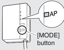
**2** Connect the smartphone (tablet PC) directly with the adapter via Wireless LAN.
