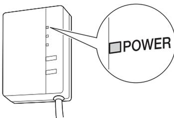
◆ When turning on the power, always attach the adapter case (upper).
